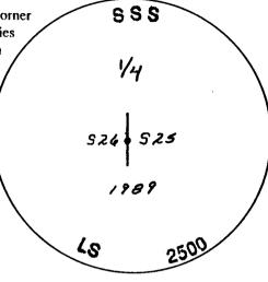
Set 5/8" x 24" long Rebar with 2" aluminum cap stamped as shown, set from reference monument 40.00' east of corner position, monument lying 0.4' feet below gravel road surface.
